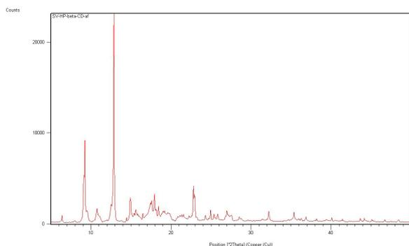
The powder X-ray diffraction pattern of SV-β-CD co-precipitation inclusion complex shown the presence of a new compound with a lot of β-CD characteristics, but still maintaining some of SV peaks.
