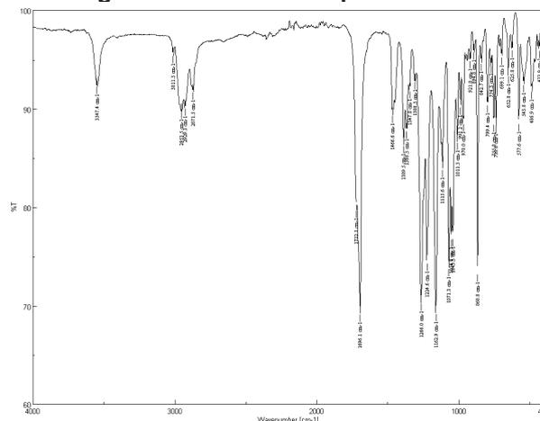
The FT-IR spectra of  $\beta$ -CD (figure 18) showed a large absorption band at 3314  $\text{cm}^{-1}$  (O-H stretching vibrations), 2924  $\text{cm}^{-1}$  (C-H stretching vibrations) and at 1021  $\text{cm}^{-1}$  a very strong band produced by the C-O bond's vibration.
