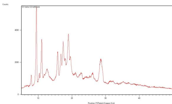
The SV - HP-β-CD lyophilization inclusion complex presented the powder X-ray diffraction pattern with less peaks low intensity, keeping somehow the base characteristics of the initial substances, but a new system with an amorphous structure was formed.
