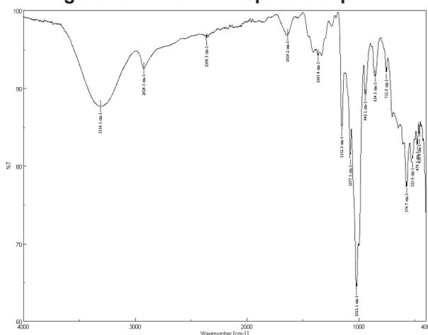
The FT-IR spectra of SV- $\beta$ -CD physical mixture (figure 19) is the arithmetic sum of IR spectra of the components, without changes in the wavelengths of spectra's maximum.
