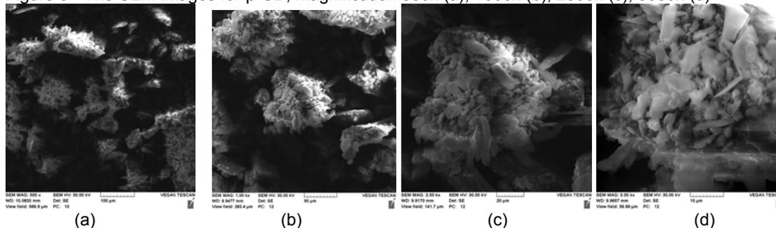
$\beta$ -CD has, also, different shapes of crystalline particles, with homogenous surface, with sizes between 5 and 10 an 10  $\mu\text{m}$ .
