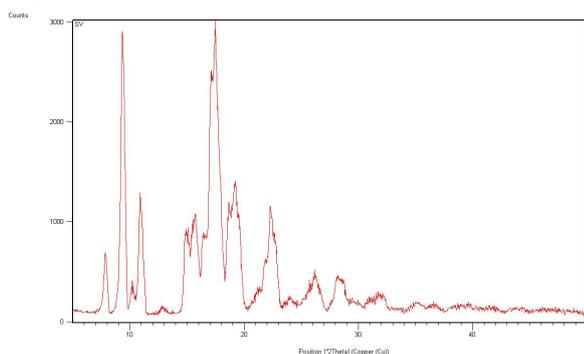
The powder X-ray diffraction pattern of SV shows that the drug is present as a crystalline form, by the presence of several distinct peaks at a  $2\theta$  diffraction angle of  $7,87^\circ$ ,  $9,31^\circ$ ,  $10,98^\circ$ ,  $12,86^\circ$ ,  $15,61^\circ$ ,  $16,49^\circ$ ,  $17,28^\circ$ ,  $18,85^\circ$ ,  $22,56^\circ$ ,  $25,93^\circ$ ,  $28,37^\circ$  și  $31,94^\circ$ .
