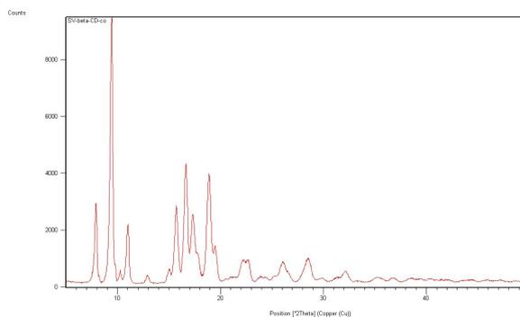
The powder X-ray diffraction pattern of SV- $\beta$ -CD physical mixture presents the overlap of the spectra registered for both components, not showing the formation of a new compound with a new structure. Yet, the powder X-ray diffraction pattern of the physical mixture is more like the one corresponding to SV.
