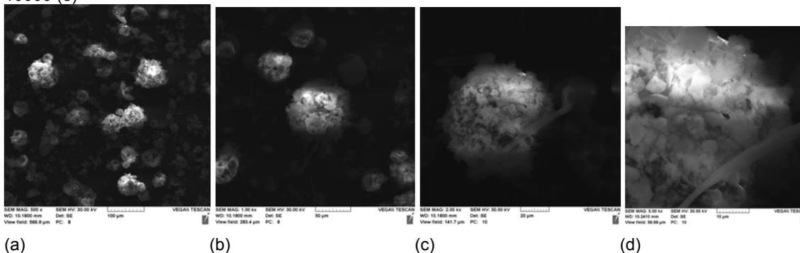
The SEM images for the SV-  $\beta$ -CD physical mixture clearly shown the crystalline structures of SV and  $\beta$ -CD, but the crystals of drug and the particles of CD were seen adhering to their surface, this confirming the affinity between substrates.
