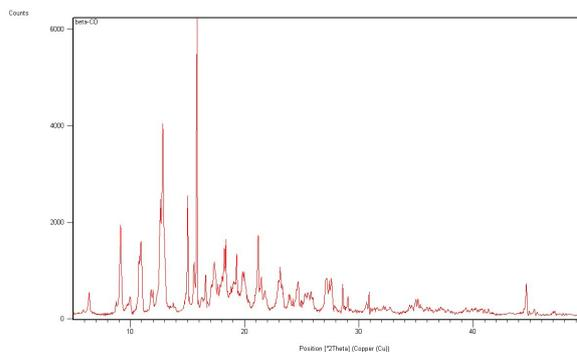
The presence of a series of intense peaks in the powder X-ray diffraction pattern of  $\beta$ -CD also indicates the fact that the substance has a crystalline nature.
